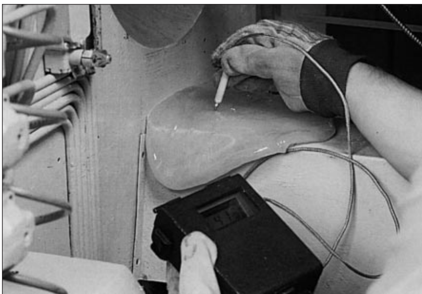
Figure 15 Making an Accurate Melt Temperature Reading
