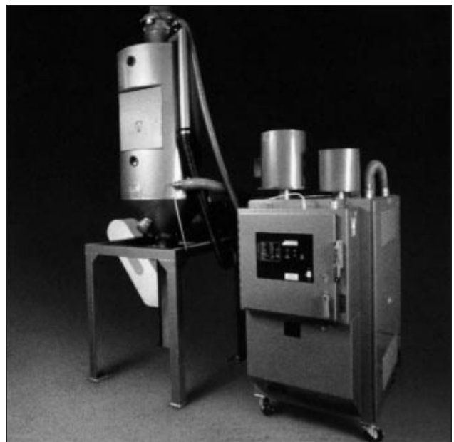
Figure 11 Typical Desiccant Dehumidifying Hopper Dryer System
