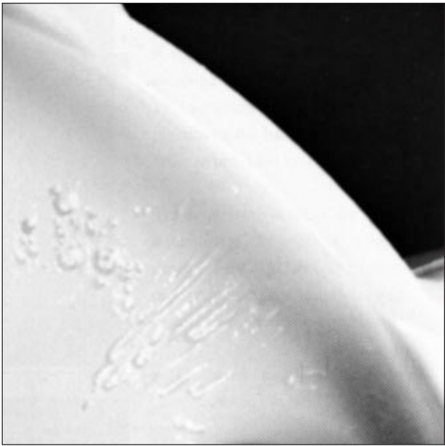
Figure 27 Blister and Splay Marks
